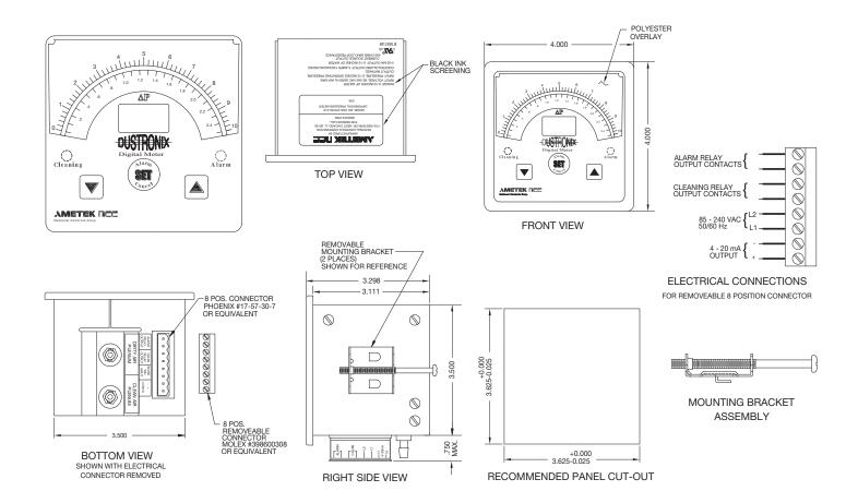
Accuracy: ±2% of full scale at 77°F (25°C); ±5% of full scale over temperature and voltage range Maximum Continuous Pressure: 10 psi
